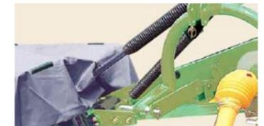
In mowing operation, cutting level must be kept evenly in the range of cutting width. 2 suspension springs work as the top and bottom edges keep the same level and follow the ground.
