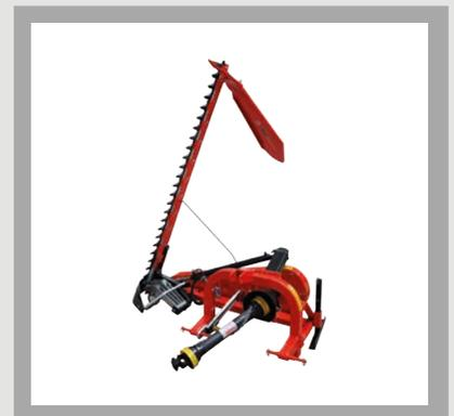
Agromaster Sickle Bar Mower is mounted to tractors by three point Linkage system and operated by PTO of tractor. By the help of tooth-blade motion system it makes possible a scissors cut which leads to a high speed operation on any crop. Also tooth-blade motion guarantees a sharp and clean cut on any type of grass, be it wet or flattened.
