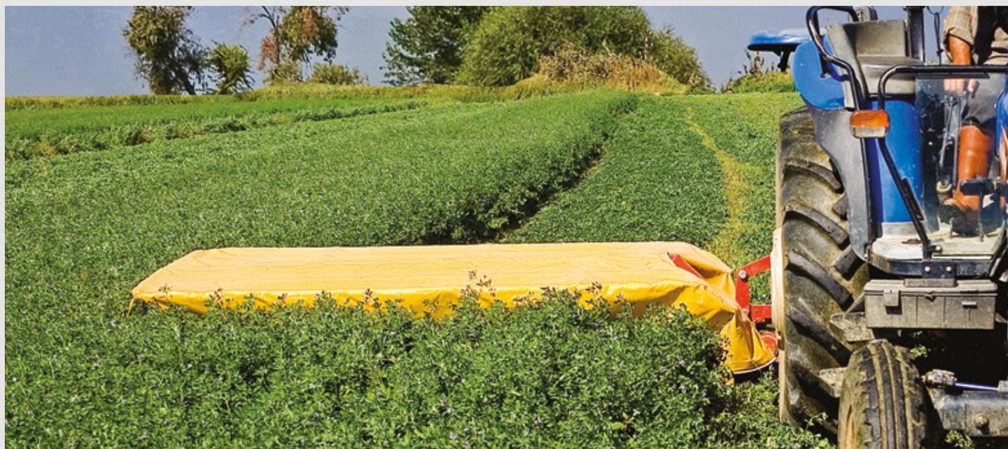
Rotary mower TOB is used to cut grass, meadow grass, feed plants with blades rotating at a high speed existing on both of the 2 drums rotating reversely to each other. Cutting height adjusting function and high quality cutting provides to keep nutrient values of plants and drying is made possible in a short time. By means of safety mechanism the machine is protected against damage which may occur if it hits hard and big objects (tree, stone, etc.), by moving backward.
