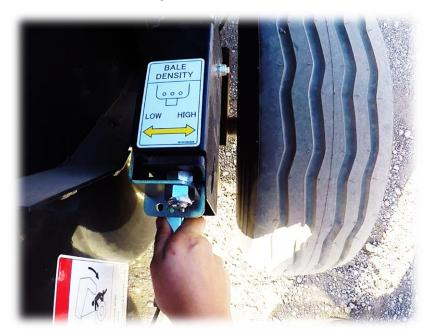
This baler requires little skill to operate. Just wait for the horn on the control box to sound, then stop moving forward, turn and watch the roll of net wrap. When the roll of net wrap stops turning, the bale is complete and ready to be discharged from the baler.
