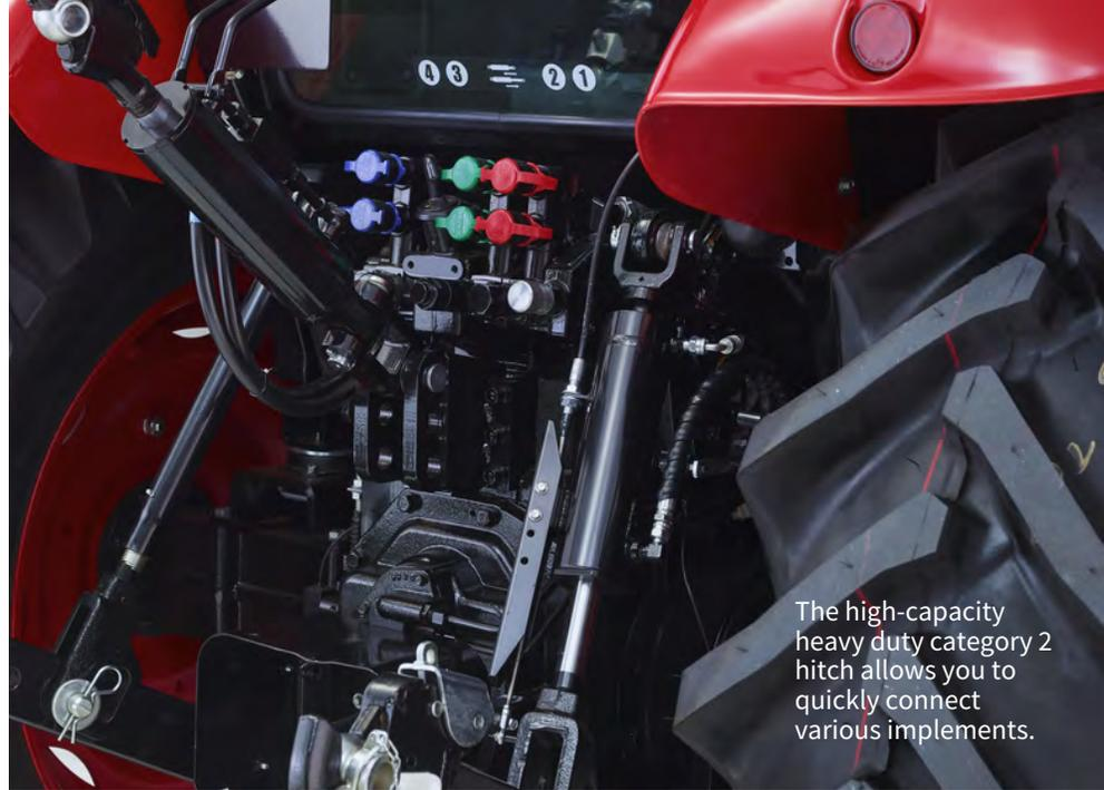
The high-capacity heavy-duty category 2 hitch allows you to quickly connect various implements.
