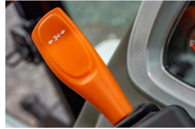
The shuttle lever on TYM tractors provides operators with precise control for quick and seamless directional changes needed for loader work, mowing, plowing, and more.
