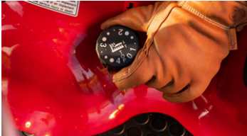
6. Dial adjustment for mower height
