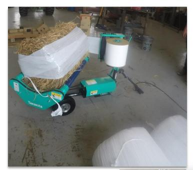
The Takakita WM511 runs on any 110-voltage outlet. It can wrap over 100 bales per hour in average conditions.
